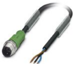
Sensor/actuator cable, 3-position, PUR halogen-free, black-gray RAL 7021, Plug straight M12, coding: A, on free cable end, cable length: 10 m
