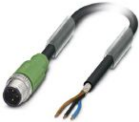
Sensor/actuator cable, 3-position, PUR halogen-free, black-gray RAL 7021, shielded, Plug straight M12, coding: A, on free cable end, cable length: 3 m
