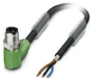
Sensor/actuator cable, 3-position, PUR halogen-free, black-gray RAL 7021, shielded, Plug angled M12, coding: A, on free cable end, cable length: 1.5 m
