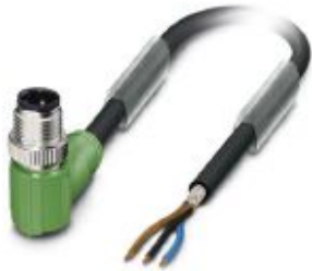
Sensor/actuator cable, 3-position, PUR halogen-free, black-gray RAL 7021, shielded, Plug angled M12, coding: A, on free cable end, cable length: 3 m
