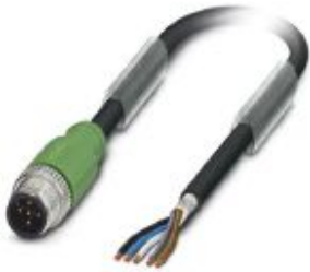
Sensor/actuator cable, 5-position, PUR halogen-free, black-gray RAL 7021, shielded, Plug straight M12, coding: A, on free cable end, cable length: 5 m
