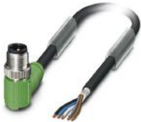
Sensor/actuator cable, 5-position, PUR halogen-free, black-gray RAL 7021, shielded, Plug angled M12, coding: A, on free cable end, cable length: 3 m
