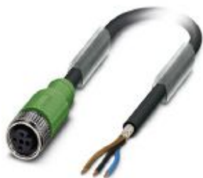
Sensor/actuator cable, 3-position, PUR halogen-free, black-gray RAL 7021, shielded, free cable end, on Socket straight M12, coding: A, cable length: 3 m
