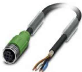
Sensor/actuator cable, 4-position, PUR halogen-free, black-gray RAL 7021, shielded, free cable end, on Socket straight M12, coding: A, cable length: 1.5 m
