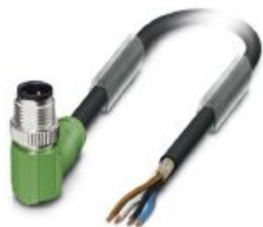
Sensor/actuator cable, 4-position, PUR halogen-free, black-gray RAL 7021, shielded, Plug angled M12, coding: A, on free cable end, cable length: 1.5 m
