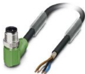
Sensor/actuator cable, 4-position, PUR halogen-free, black-gray RAL 7021, shielded, Plug angled M12, coding: A, on free cable end, cable length: 5 m
