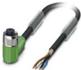
Sensor/actuator cable, 4-position, PUR halogen-free, black-gray RAL 7021, shielded, free cable end, on Socket angled M12, coding: A, cable length: 5 m
