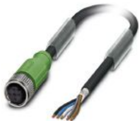
Sensor/actuator cable, 5-position, PUR halogen-free, black-gray RAL 7021, shielded, free cable end, on Socket straight M12, coding: A, cable length: 1.5 m
