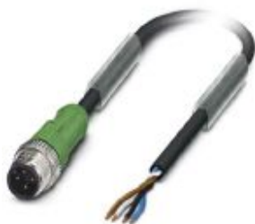
Sensor/actuator cable, 4-position, PUR halogen-free, black-gray RAL 7021, Plug straight M12, coding: A, on free cable end, cable length: 10 m
