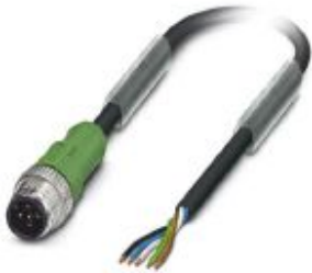
Sensor/actuator cable, 5-position, PUR halogen-free, black-gray RAL 7021, Plug straight M12, coding: A, on free cable end, cable length: 10 m
