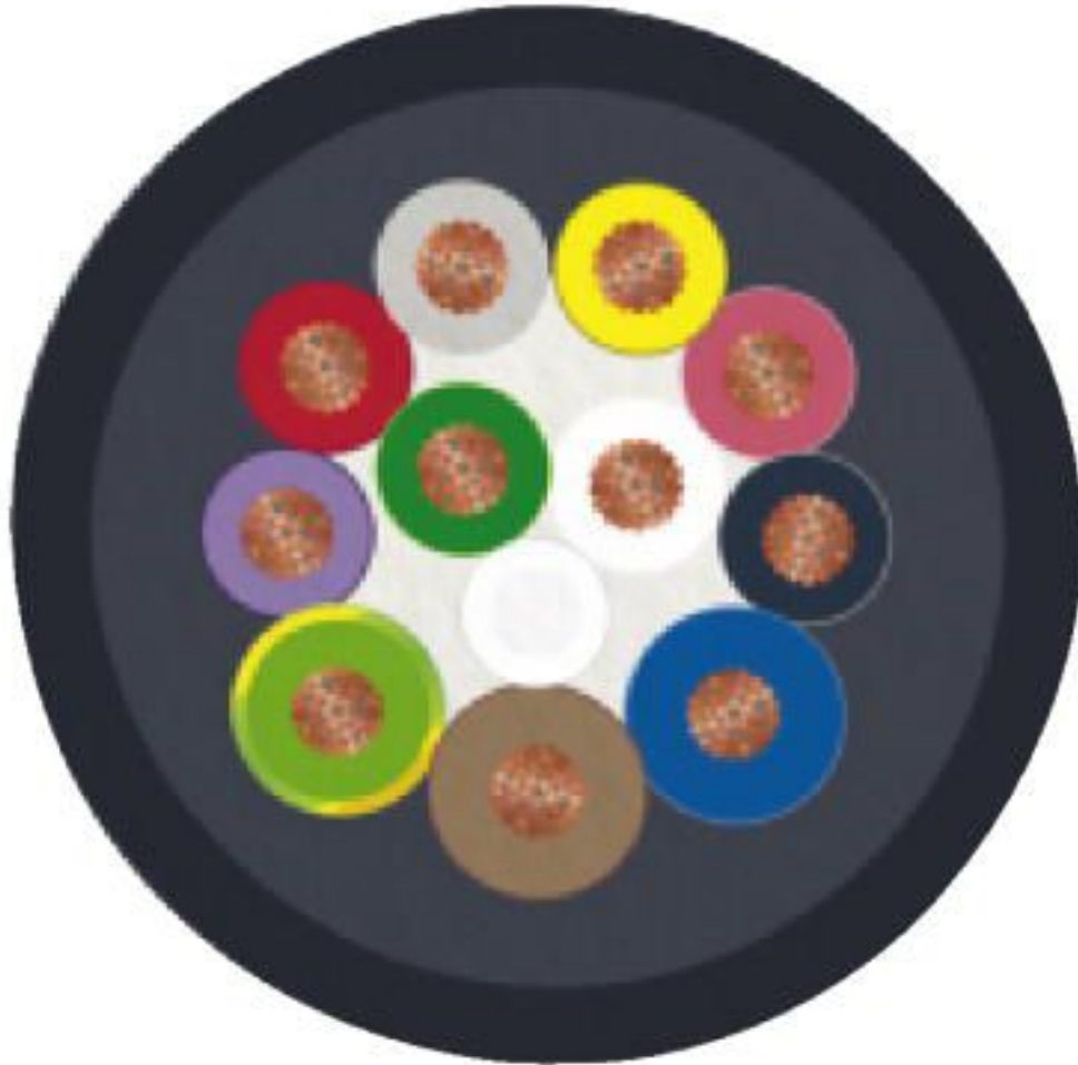
Cable cross section
