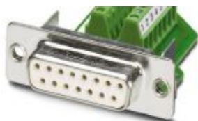
D-SUB contact insert, shell size 2, with 15 signal contacts, female type of contact, screw connection, straight, for panel mounting frame and sleeve housing with IP67 protection
