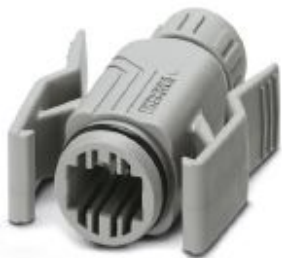
RJ45 sleeve housing, IP67, for pin insert VS-08-ST-RJ45, with push-pull interlocking for panel mounting frames, for cable cross section 5.0 mm ... 6.5 mm
