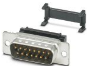
D-SUB contact insert, shell size 2, with 15 signal contacts, type of contact pin, flat-ribbon cable connection, angled, fixing with a 3 mm hole, for panel mounting frame VS-15-...
