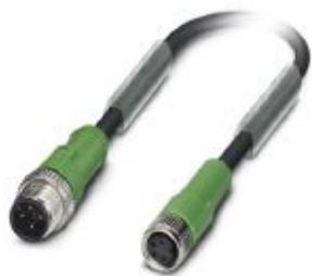
Sensor/actuator cable, 4-position, PUR halogen-free, black-gray RAL 7021, Plug straight M12, coding: A, on Socket straight M8, coding: A, cable length: 1.5 m
