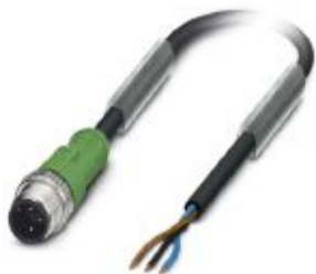
Sensor/actuator cable, 3-position, PVC, black RAL 9005, Plug straight M12, coding: A, on free cable end, cable length: 5 m
