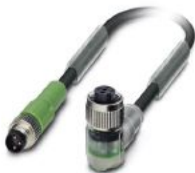
Sensor/actuator cable, 3-position, PUR halogen-free, black-gray RAL 7021, Plug straight M8, on Socket angled M12, coding: A, with 2 LEDs, cable length: 3 m
