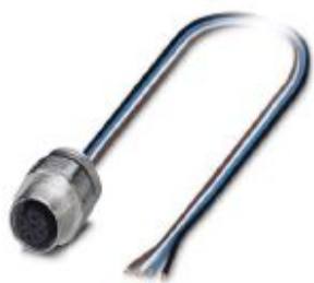
Sensor/Actuator flush-type socket, 4-pos., M12, A-coded, front/screw mounting with Pg9 thread, can be positioned, with 0.5 m TPE litz wire, 4x 0.34 mm 2
