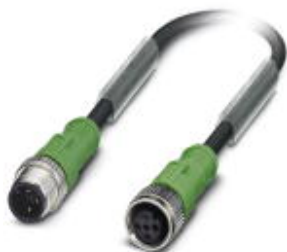
Sensor/actuator cable, 3-position, PUR halogen-free, black-gray RAL 7021, Plug straight M12, A-coded, on Socket straight M12, A-coded, cable length: 10 m
