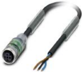
Sensor/actuator cable, 3-position, PUR halogen-free, black-gray RAL 7021, free cable end, on Socket straight M12, coding: A, with 2 LEDs, cable length: 1.5 m
