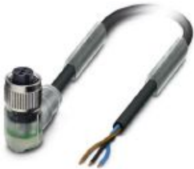
Sensor/actuator cable, 3-position, PUR halogen-free, black-gray RAL 7021, free cable end, on Socket angled M12, coding: A, with 2 LEDs, cable length: 10 m
