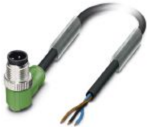
Sensor/actuator cable, 3-position, PUR halogen-free, black-gray RAL 7021, Plug angled M12, coding: A, on free cable end, cable length: 10 m
