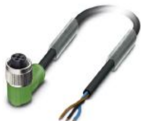
Sensor/actuator cable, 3-position, PUR halogen-free, black-gray RAL 7021, free cable end, on Socket angled M12, coding: A, cable length: 3 m
