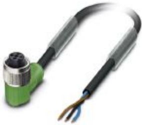
Sensor/actuator cable, 3-position, PUR halogen-free, black-gray RAL 7021, free cable end, on Socket angled M12, coding: A, cable length: 10 m
