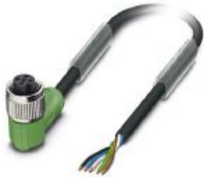
Sensor/actuator cable, 5-position, PUR halogen-free, black-gray RAL 7021, free cable end, on Socket angled M12, coding: A, cable length: 10 m
