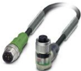
Sensor/actuator cable, 5-position, PUR halogen-free, black-gray RAL 7021, Plug straight M12, coding: A, on Socket angled M12, coding: A, with 3 LEDs, cable length: 0.3 m
