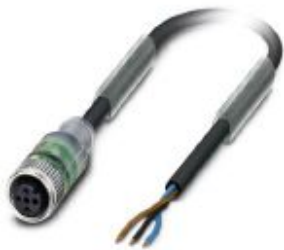
Sensor/actuator cable, 3-position, PUR halogen-free, black-gray RAL 7021, free cable end, on Socket straight M12, coding: A, with 2 LEDs, cable length: 10 m
