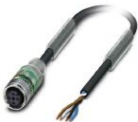
Sensor/actuator cable, 4-position, PUR halogen-free, black-gray RAL 7021, free cable end, on Socket straight M12, coding: A, with 2 LEDs, cable length: 1.5 m
