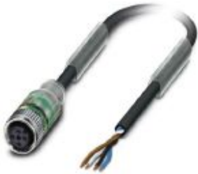
Sensor/actuator cable, 4-position, PUR halogen-free, black-gray RAL 7021, free cable end, on Socket straight M12, coding: A, with 2 LEDs, cable length: 3 m
