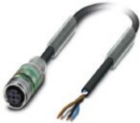
Sensor/actuator cable, 4-position, PUR halogen-free, black-gray RAL 7021, free cable end, on Socket straight M12, coding: A, with 2 LEDs, cable length: 5 m
