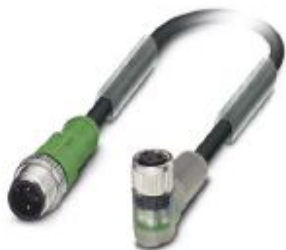
Sensor/actuator cable, 3-position, PUR halogen-free, black-gray RAL 7021, Plug straight M12, coding: A, on Socket angled M8, with 2 LEDs, cable length: 3 m
