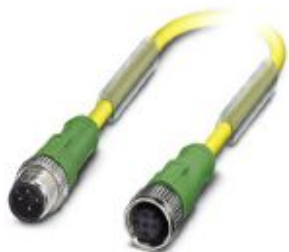
Sensor/actuator cable, 4-position, PUR/PVC, yellow, Plug straight M12, coding: A, on Socket straight M12, coding: A, cable length: 0.3 m, DESINA
