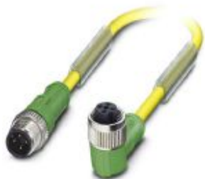
Sensor/actuator cable, 4-position, PUR/PVC, yellow, Plug straight M12, coding: A, on Socket angled M12, coding: A, cable length: 0.6 m, DESINA
