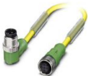
Sensor/actuator cable, 4-position, PUR/PVC, yellow, Plug angled M12, coding: A, on Socket straight M12, coding: A, cable length: 1.5 m, DESINA
