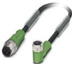
Sensor/actuator cable, 4-position, Variable cable type, Plug straight M12, coding: A, on Socket angled M8, cable length: Free input (0.2 ... 40.0 m)
