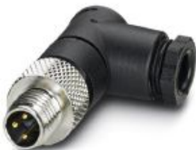
Connector, Universal, 3-position, Plug angled M8, Coding: A, Solder connection, knurl material: Nickel-plated brass, external cable diameter 3.5 mm ... 5 mm
