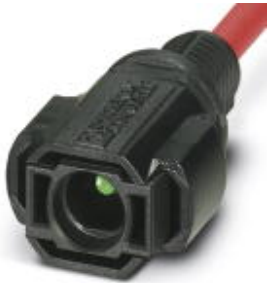
Photovoltaic connector, Photovoltaic connector, color: black, Min. wire cross section: 4, Connection method: Crimp, Type of contact: Pin, Cable length: 300. can only be released using a tool
