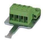
PCB connector, nominal current: 76 A, rated voltage (III/2): 1000 V, nominal cross section: 16 mm², number of positions: 3, pitch: 10.16 mm, connection method: Screw connection with tension sleeve, color: green, contact surface: Silver
