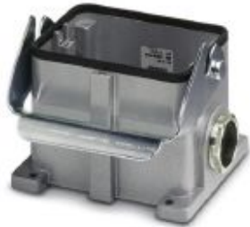
Box mounting base, with single locking latch, height 100 mm, with screw connection, 2x Pg29
