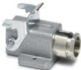
HEAVYCON D7 box mounting base, with single locking latch, height 25.5 mm, with 1 x Pg11 screw connection, with open bottom, zinc
