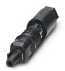
Photovoltaic connector, Range of articles: PV-CF-S, Connector, housing material: PPE, color: black, number of positions: 0, min. conductor cross section: 6 mm², max. conductor cross section: 16 mm², rated current: 40 A, Connection method: Spring-cage, Type of contact: Socket
