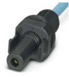
Photovoltaic connector, Photovoltaic connector, housing material: PPE, color: black, number of positions: 1, min. conductor cross section: 6 mm<sup>2</sup>, Connection method: Crimp, Type of contact: Socket, cable length: 130
