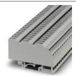
Feed-through terminal block, nom. voltage: 800 V, nominal current: 20 A, connection method: Screw/plug-in connection, number of connections: 4, number of positions: 1, cross section: 0.2 mm² - 4 mm², AWG: 24 - 12, width: 7.6 mm, color: gray, mounting type: NS 35/7,5, NS 35/15, NS 32
