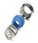
EMC half screw connection Pg21, for metal housings of sizes 2-4, consisting of rubber seal, iris spring, cone disks and pressure screw, for size 1 housings, cable shielding range [mm] 10.5 - 14.5, cable [mm] 14-18
