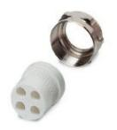
Single screw connection Pg21, made of metal, consisting of rubber seal with a long hole and pressure screw, for type 2-4 housings, cable [mm] 20 x 7 mm (for flat-ribbon cable)
