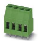
PCB terminal block, nominal current: 24 A, rated voltage (III/2): 400 V, nominal cross section: 2.5 mm², pitch: 5 mm, number of positions: 8, connection method: Screw connection with tension sleeve, mounting: Wave soldering, conductor/PCB connection direction: 0 °, color: green, Pin layout: Linear pinning, Solder pin [P]: 3.6 mm. The article can be aligned to create different nos. of positions!
